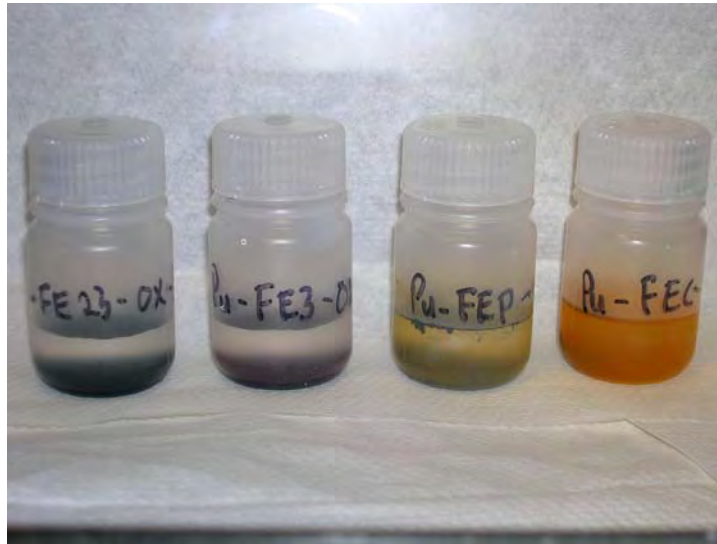
Figure 4-10. Appearance of Pu-Fe experiments after reaction. Experiments above were (left to right): Magnetite in ERDA-6, Ferrite in ERDA-6 brine, iron powder in ERDA-6 brine, and iron coupon in ERDA-6 brine
